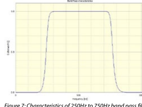
Figure 7: Characteristics of 250Hz to 750Hz band pass filter
