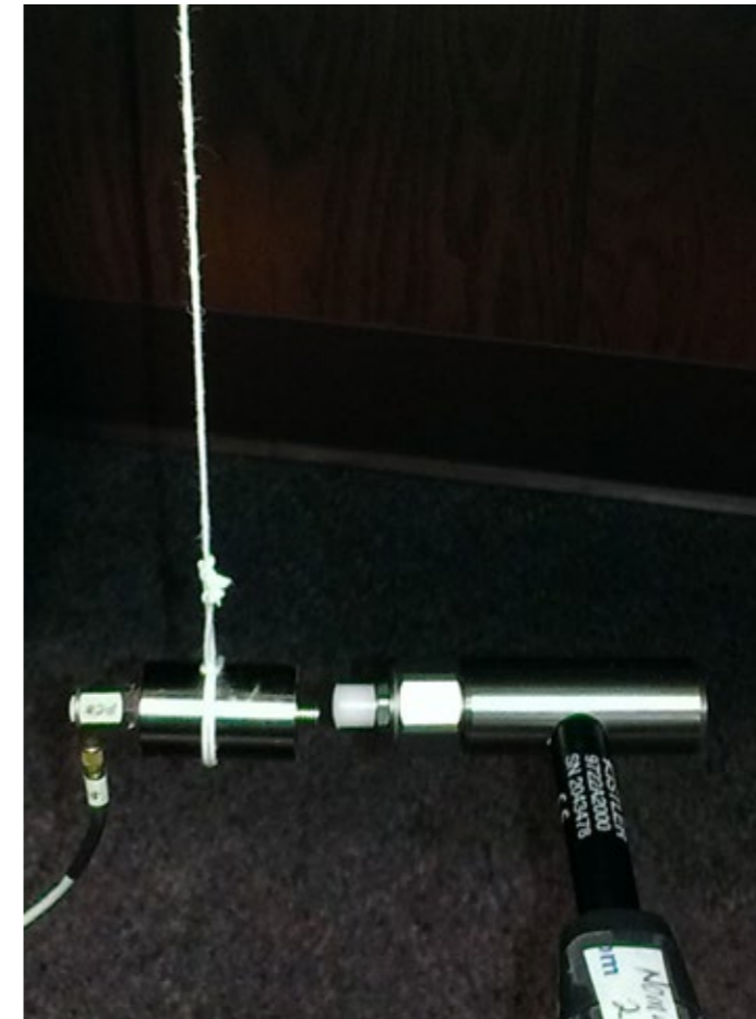
Figure 2: Improvised system to calibrate an impact hammer
